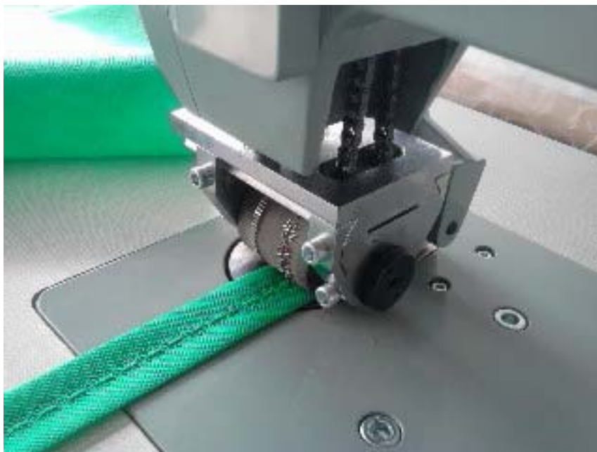
B. YDN-50-D press machine. This machine is used to weld the sleeve handles onto the mouth of the bags.
