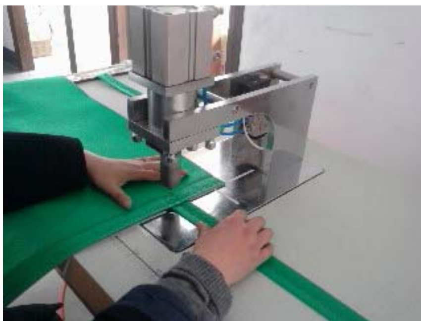
B. YDN-50-D press machine. This machine is used to weld the sleeve handles onto the mouth of the bags.
