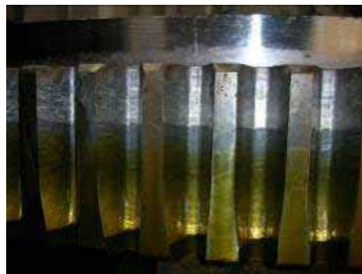
Gears being cut
