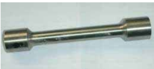
Material cut from the rings for tensile test
