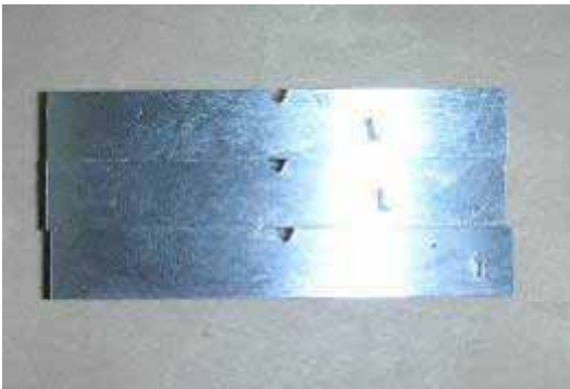
Material cut from the rings for impact test
