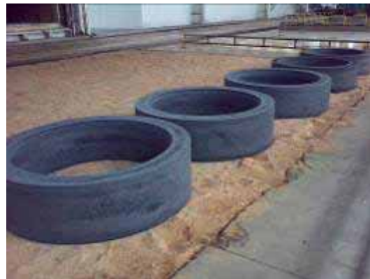
Forged rings after heating treatment
