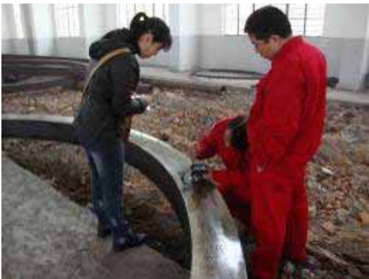
Hardness test to the forged rings
