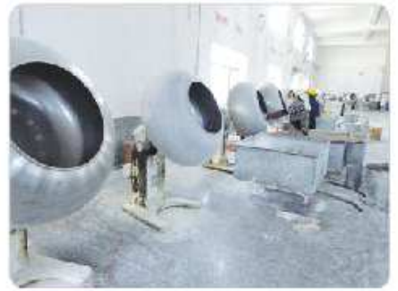
搪球 Production of Ceramic Balls
